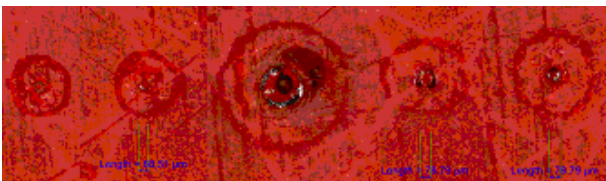
Fig 9: Polymeric material AF 163 showing signs of thermal damage, surrounding the holes..
