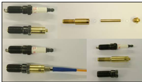
Figure 4. Photographs of the optical plug: disassembled, with optical fibre attached and compared with a conventional spark plug.
