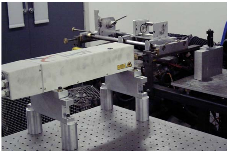
Figure 5. The laser off the engine with the optics on the engine. The final focusing lens cannot be seen as it is in the cylinder
