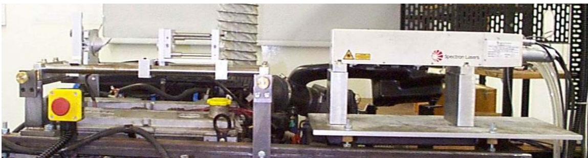
Figure 2. Photograph of the laser and optics on the engine. The final focusing lens cannot be seen as it is in the cylinder
