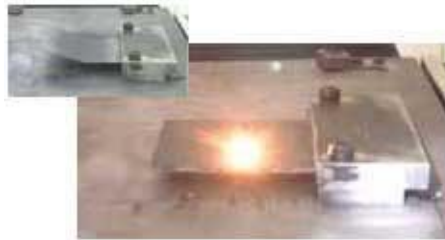
Figure 1. The laser forming process on 2mm Ti6Al4V using 800W CO 2 laser power and a 6mm beam diameter.
