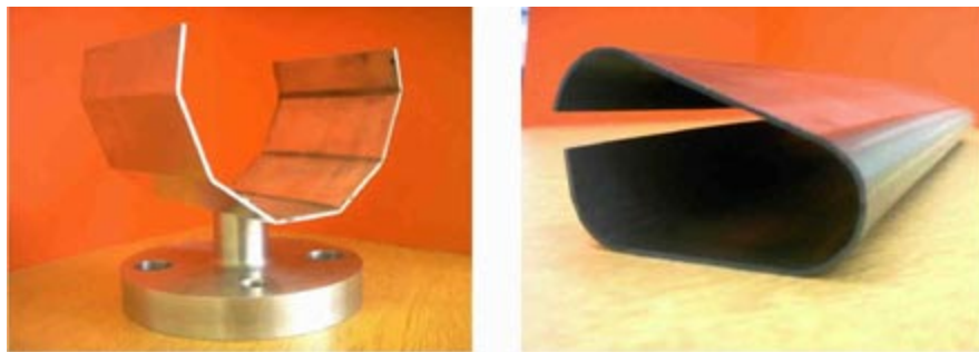
Fig. 2: Two examples of laser-formed parts. The part at left was formed from a 250 x 100 mm, 2-mm gauge aluminum blank; the other was from 400 x 200 mm, 1.5-mm gauge mild steel. Both were formed from flat sheet with no additional tooling or restraint (save the attachment to the CNC bed).
