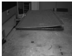
Fig. 4: Laser forming a part-cylinder along the longitudinal X axis from 800x400x5 mm mild steel sheet (height measurements along the two shorter Y axis edges)
