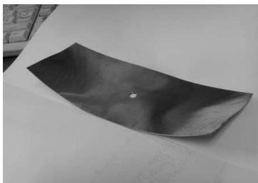
Figure 7 Final shape of 200x80mm AA5251 component (200W laser power).
