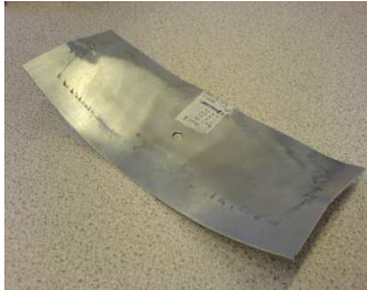
Figure 6 Final shape of 200x80mm AA5251 component (400W laser power).
