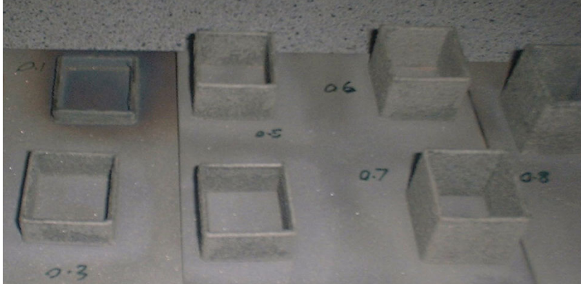
Fig. 4: Square structures built with different layer heights under constant deposition parameters. Each square is 2cm on a side.
