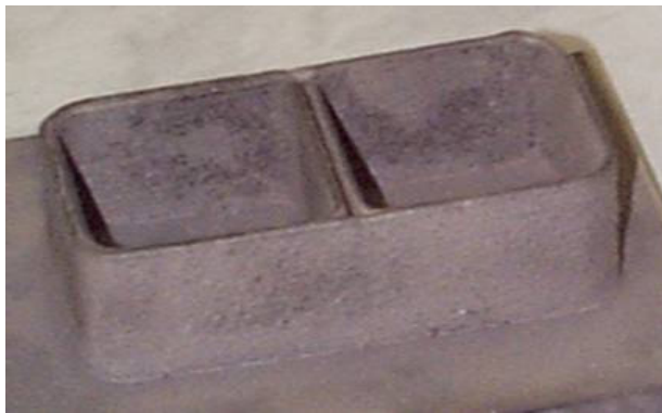
Fig.12 An example of overlapping layers height control
