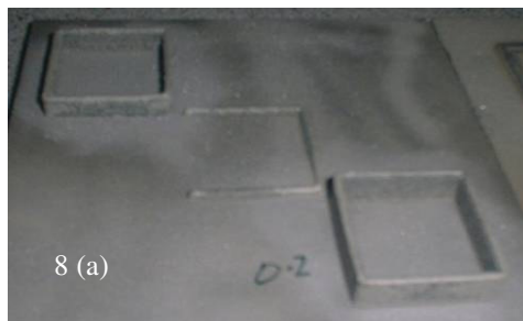
Fig.8 (a-d). Photograph 8(a) showing the first two 30 layer structures and a single first layer for purposes of assessing the initial nozzle position in relation to the substrate. This first layer is larger than the input step height due to the nozzle position being such that the top of the powder cloud is not coincident with the surface of the substrate. The total series consisted of using input step heights from 0.1 to 1.5mm in 0.1mm increments. Further examples along the run follow (anticlockwise from left: 8(b-d)) until height control failure at 1.5mm layer height
