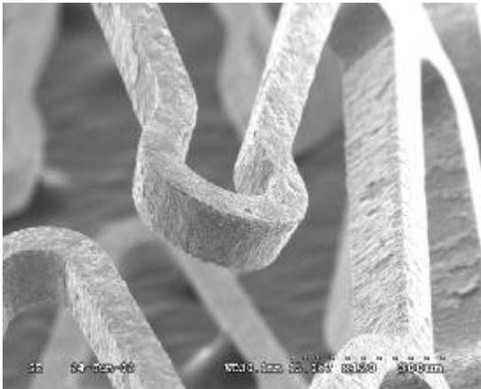
Fig. 2: SEM picture of a stainless steel stent after ultrasonic cleaning
