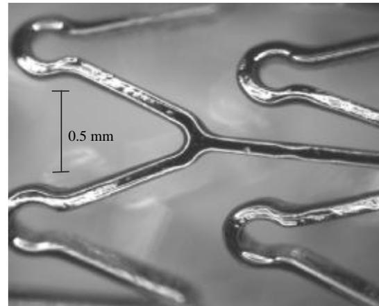
Fig. 3: Stainless steel stent after electro-polishing
