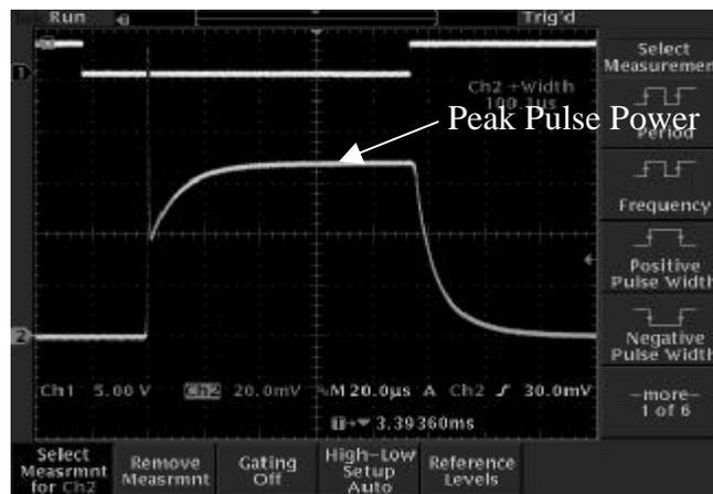
Fig. 5: Typical fiber laser pulse shape
