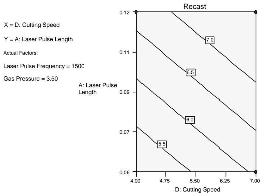
Fig. 12: Influence of laser pulse length and cutting speed on recast layer thickness (in  $\mu\text{m}$ ) at 3.5 bar assist gas pressure.
