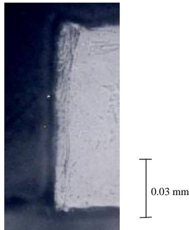
Fig. 10: Cross-section of etched stainless steel sample. The recast layer is visible on the left side of the sample.
