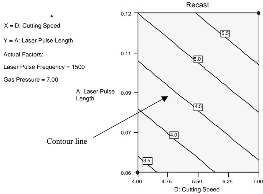
Fig. 11: Influence of laser pulse length and cutting speed on recast layer thickness (in  $\mu\text{m}$ ) at 7 bar assist gas pressure. The recast layer thickness is labeled on the contour line.
