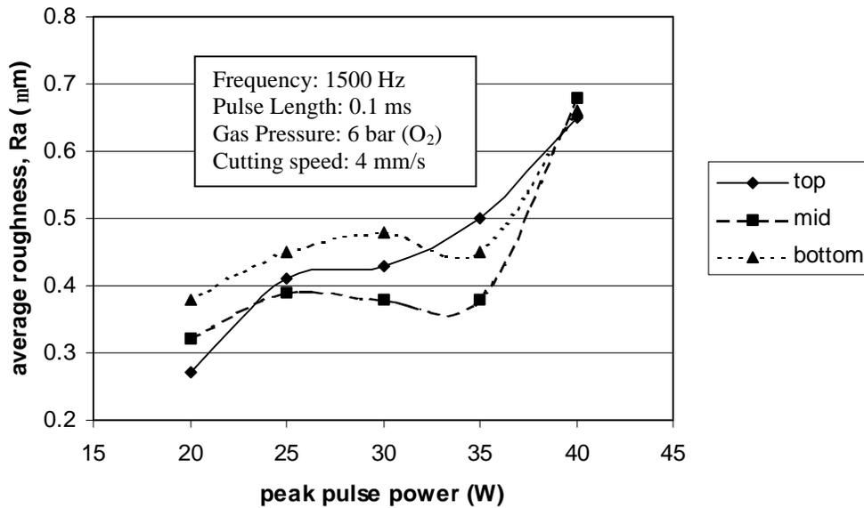
Fig. 6: Average surface roughness as function of peak pulse power
