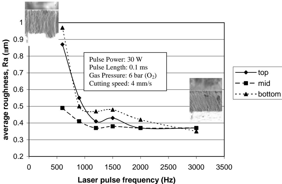
Fig. 9: Average roughness as a function of laser pulse frequency. SEM pictures for 600 Hz and 3000 Hz.
