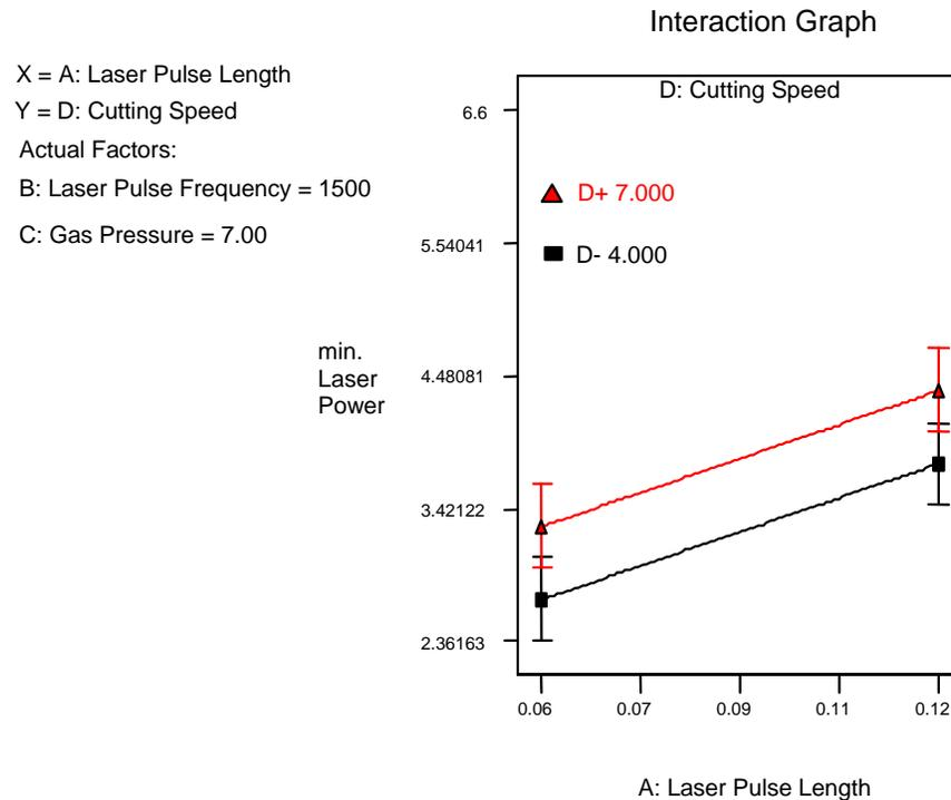
Fig. 13: Influence of laser pulse length and cutting speed on necessary minimum average power.
